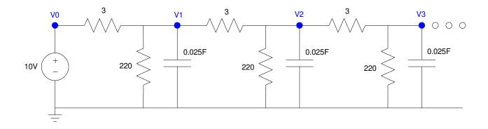
Problem 2) Write the dynamics for this system as a set of ten coupled differential equations:
