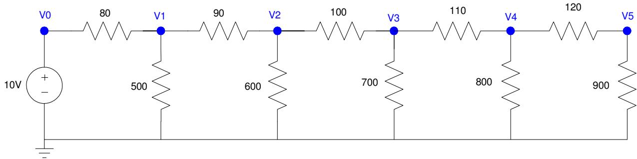
$$\left(\frac{V_1-V_0}{80}\right) + \left(\frac{V_1-V_2}{90}\right) + \left(\frac{V_1}{500}\right) = 0$$
