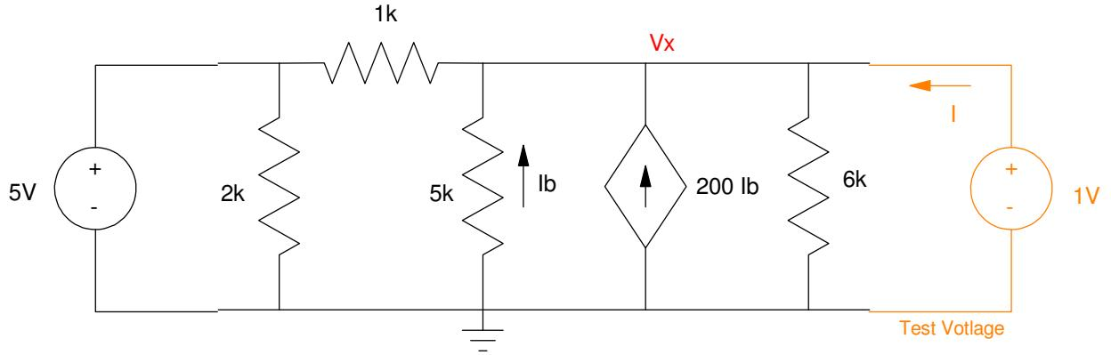
V<sub>th</sub>: Compute the open circuit voltage. To do this, write the voltage node equation at V<sub>x</sub>
