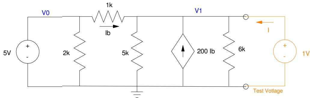
V<sub>th</sub>: Measure the open-circuit voltage. To do this, write the voltage node equation at V<sub>1</sub>
