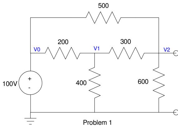
Open Circuit Voltage: Write the voltage node equations
