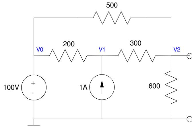
Open Circuit Voltage: Write the voltage node equations
