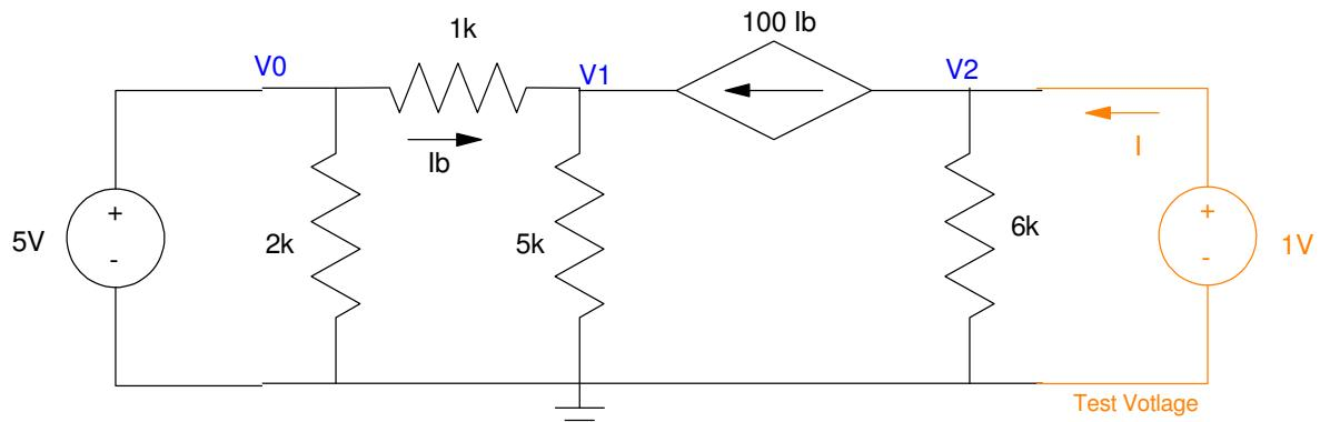
V<sub>th</sub>: Compute the open-circuit voltage. To do this, compute V<sub>1</sub>
