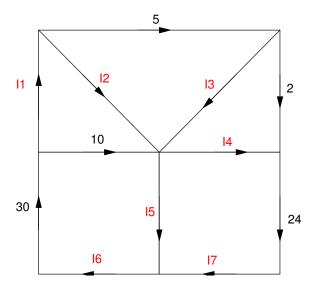
To solve for the unknown currents, find a point where there is one unknown current flowing to (or from) that node:
