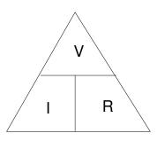
Using the passive sign-convention, V = IR, I = V/R, R = V/I
