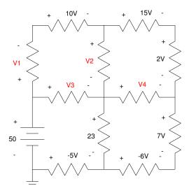
Around any closed-path, the voltages must sum to zero. Since there are five unknown voltages, if you write 4 equations you can solve for the 4 unknowns.
