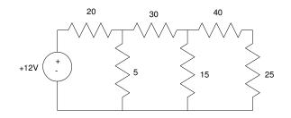
The 40 Ohm and 25 Ohm are in series. Add these to 65 Ohms.
