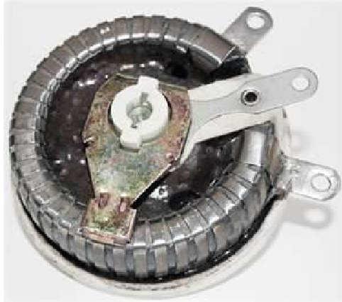
Potentiometer: A long resistive wire connects the two end terminals. A center tap lets you output the voltage or resistance in-between the end terminals. from www.westfloridacomponents.com
