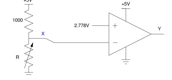
Connect the voltage divider to the negative input.
