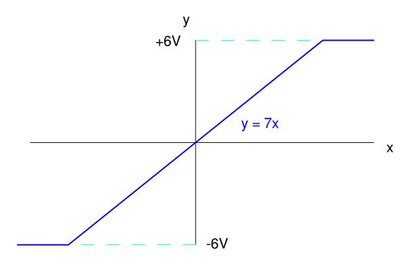
With  $\pm$ - 6V power supplies, the output (y) is limited to  $\pm$ 6V and  $\pm$ 6V
