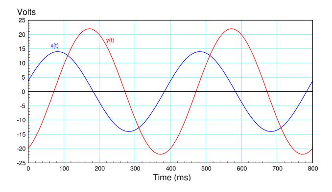
Start with the frequency: frequency is defined as cycles per second or one over the period.
