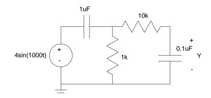
First, convert to phaser notation. In this case, due to the input being a 1000 rad/sec sine wave:
