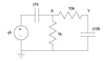
Current loops or voltage nodes work for this circuit. Selecting voltage nodes,
