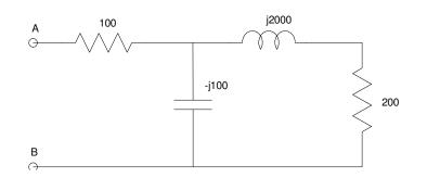
Add the resistor and inductor in series
