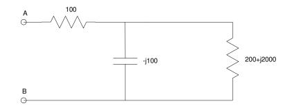
Add the capacitor in parallel with the 200+j200 impedance
