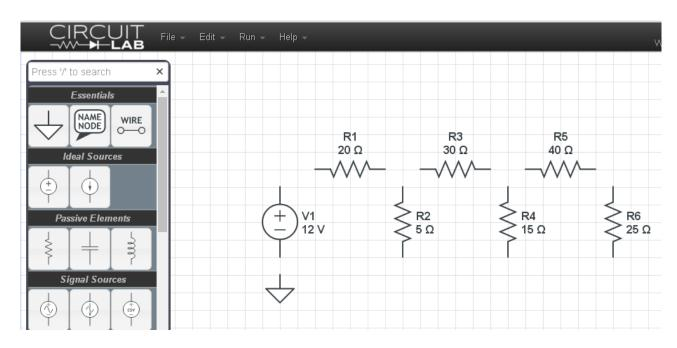
Step 2: Connect the components using drag and drop. Note: you should see a dot when wires are connected. No dot means there's no connection.
