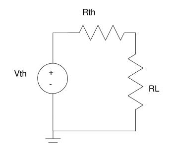
**Case 1:**  $R_{th}$  is fixed. Find  $R_L$  to maximize the power to the load.
