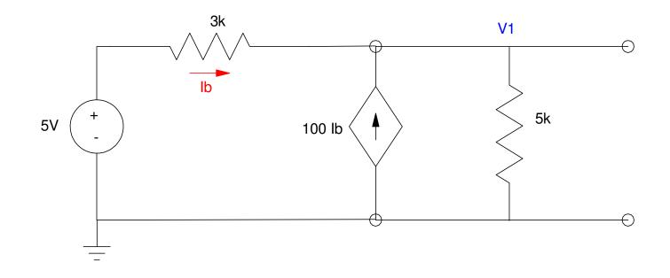
$V_{th}$ : Determine the open-circuit voltage. Write the voltage node equation at V1
