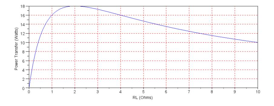
**Case 2:**  $R_L$  is fixed. Find  $R_{th}$  to maximize the power to the load.
