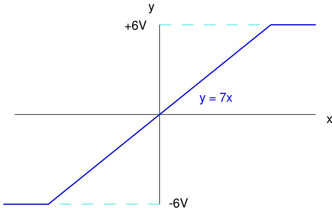
With +/- 6V power supplies, the output ( $y$ ) is limited to +6V and -6V
