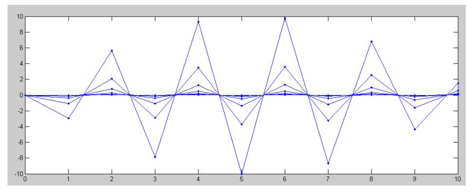
Voltages plotted every 0.05 seconds when the initial condition is the fast eigenvector
