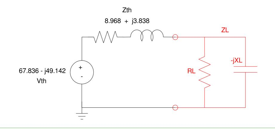
Solution: The load should be the complex conjugate of Zth
