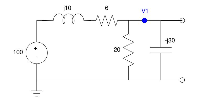
Solution: Combine the 20 Ohms and -j30 Ohms in parallel:  $20||-j30 = (13.846 - j9.231)\Omega$
