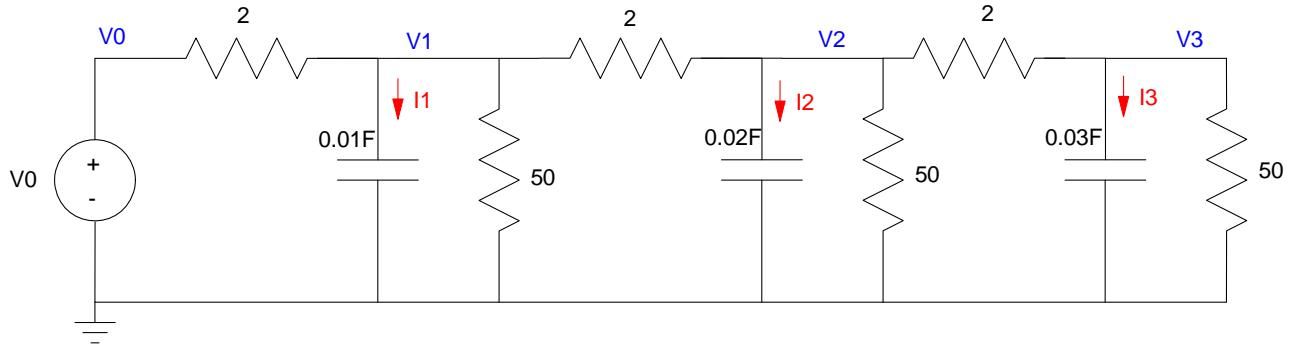
**Problem 1:** Find the transfer function from  $V_0$  to  $V_3$
