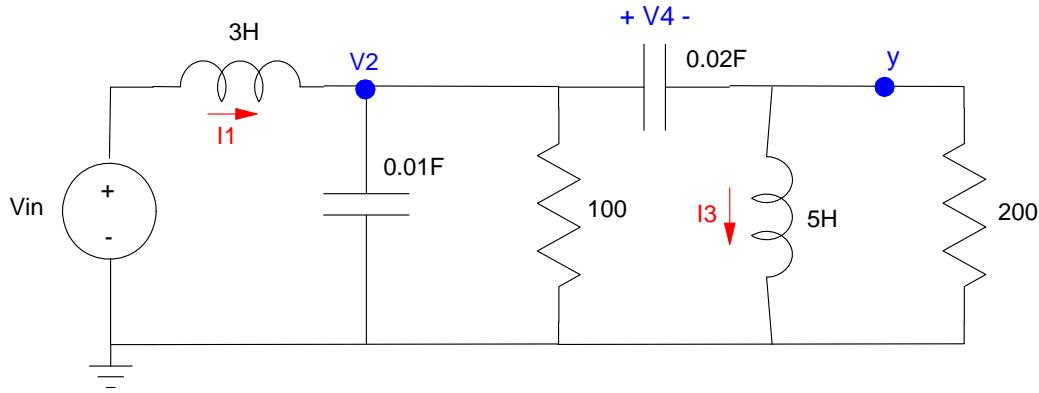
i) Write the dynamics for this system (i.e. the voltage node equations using LaPlace notation)
