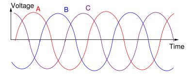
Three AC signals make up a 3-phase signal: each one 120 degrees out of phase. If you treat VA as the reference (meaning define it to be zero degree relative phase shift), then the vector diagram for these three phases then are:
