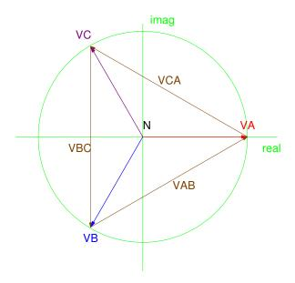
This gives the following relationship  $(V_{AN})$  means the voltage at a relative to the voltage at N, or ground):
