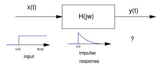
Problem: Find the output of a circuit which has an input which is not periodic.
