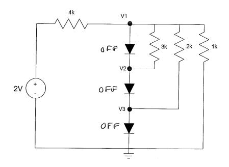
4) Assume ideal silicon diodes (Vf = 0.7V). Determine the voltages V1, V2, and V3
