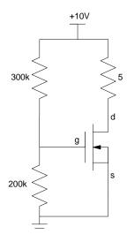
6) Draw the load line and determine the operating point if connected as shown to the right:
