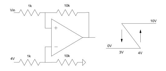
8) Schmitt Trigger: Design a circuit for a night-light which outputs
