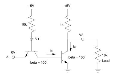
6) Determine the voltages and currents for the following TTL inverter
