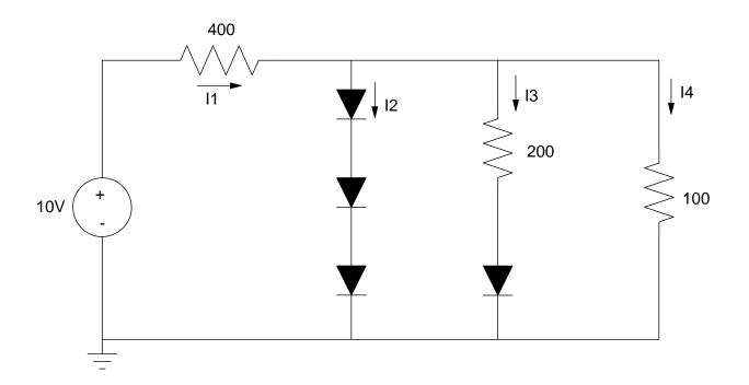
4) Assume ideal silicon diodes (Vf = 0.7V). Determine the currents, I1 - I4
