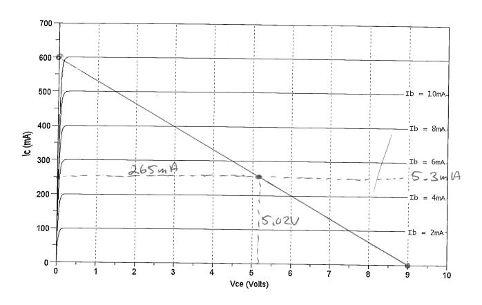
2) A transistor allows a 0V / 5V digital input to turn on and off a white LED at 100 mA.
