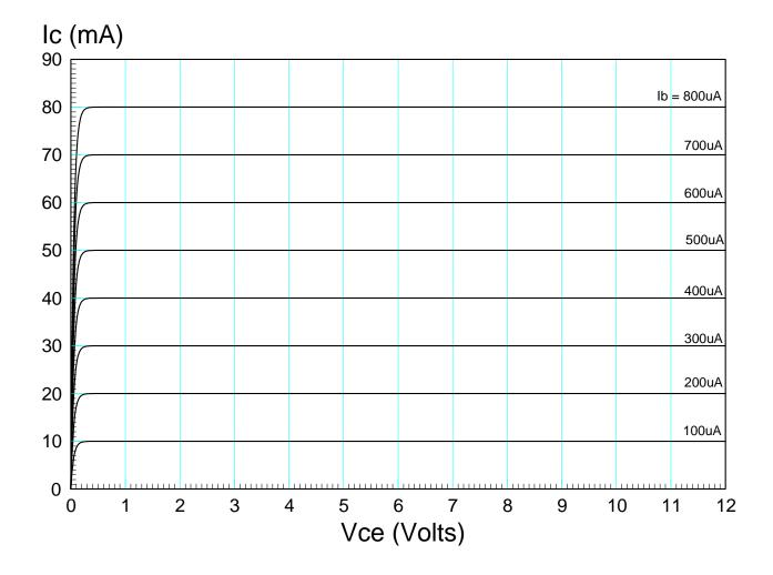
2) Draw the load line for the following circuit. Mark on the load line the operating point (termed Q-point) when
