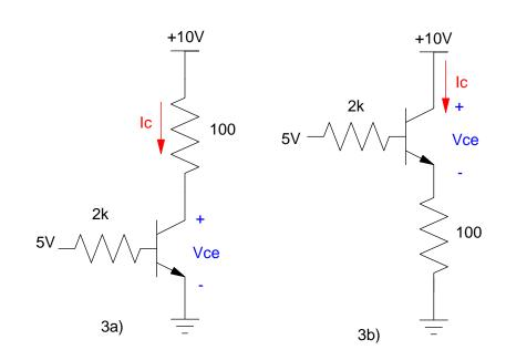
4) Design a circuit to meet the following requirements (i.e. a transistor used as a switch)
