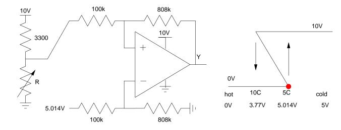
PartSim Simulation (again not necessary unless you're doing a Schmitt Trigger for your term project) PartSim crashes for positive feedback. So, use the following instead.
