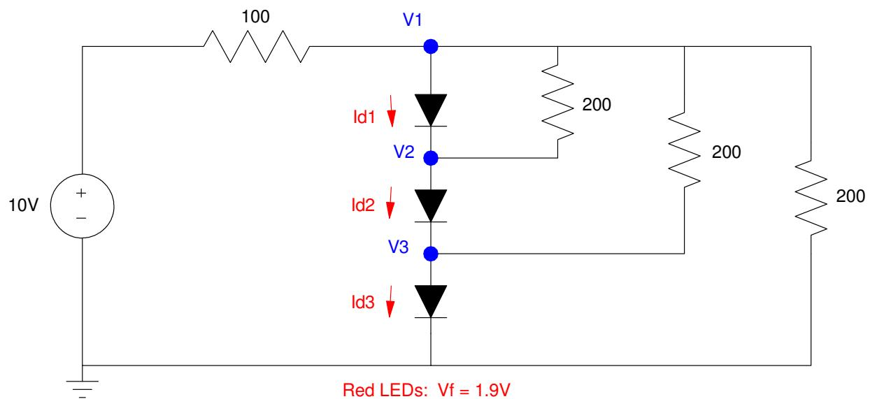
2) Determine the voltages and currents for the following circuit. Assume ideal red LEDs ( $V_f = 1.9V$ ).
