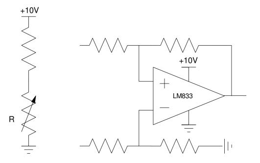
6) Schmitt Trigger: Analysis. Determine the voltages and resistance where the following Schmitt trigger turns on and off
