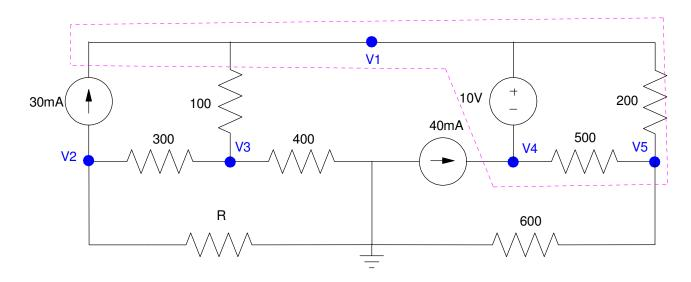
$$\begin{split} V_1 - V_4 &= 0 \\ 30mA + \left(\frac{V_2 - V_3}{300}\right) + \left(\frac{V_2}{1514}\right) &= 0 \\ \left(\frac{V_3 - V_2}{300}\right) + \left(\frac{V_3 - V_1}{100}\right) + \left(\frac{V_3}{400}\right) &= 0 \\ \left(\frac{V_5 - V_4}{500}\right) + \left(\frac{V_5}{600}\right) + \left(\frac{V_5 - V_1}{200}\right) &= 0 \\ -30mA + \left(\frac{V_1 - V_3}{100}\right) - 40mA + \left(\frac{V_5}{600}\right) &= 0 \end{split}$$
