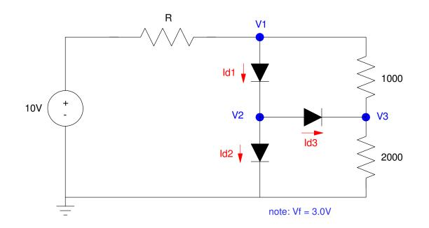
3) A red and green LED are connected to a 10V source. Determine the current and brighness of each LED. Assume
