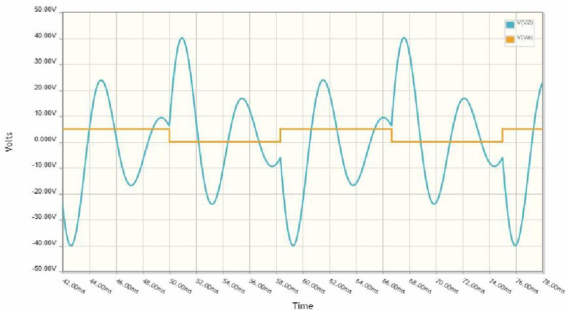
2) Adjust C1 so that the voltage across the motor is as close to a sine wave as possible (trial and error)
