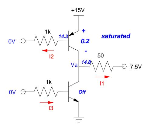
3) For the following half H-bridge, specify R1 and R2 so that the PNP transistor is saturated. Also determine the resulting currents I1 and I2. Assume the current gain is  $200 \ (\beta = 200)$
