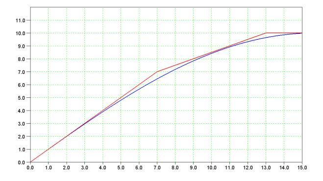
Draw in straight lines with slopes of 1, 1/2, 1/4, 1/8, etc. to approximate the curve (shown in red) Each drop in slope from 1 to 1/2 to 1/4, etc is an additional stage.
