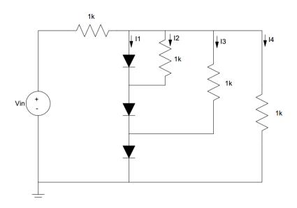
There are 3 diodes - meaning 8 permutations. One of the eight is correct (Vd < 0.7V for off diodes, Id > 0 for on diodes)
