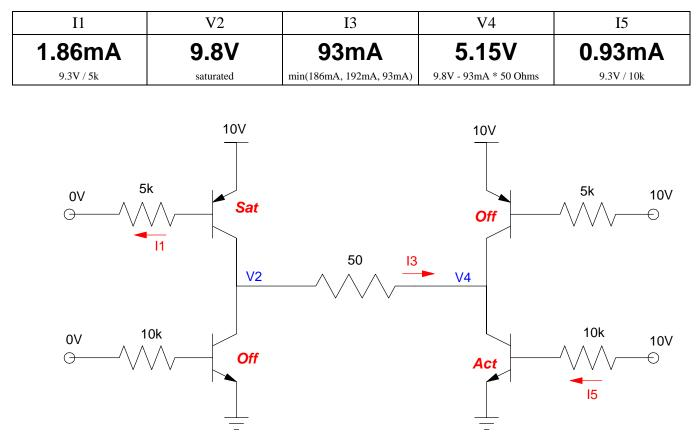
3) Assume ideal transistors with  $|V_{be}| = 0.7V$  and  $\beta = 100$ . Determine the voltages and currents.
