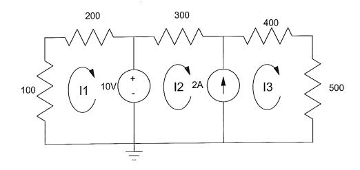
3) Write 4 current loop equations that allow you to solve for V1, V2, V3, and V4. You don't need to solve - just give the 4 equations.
