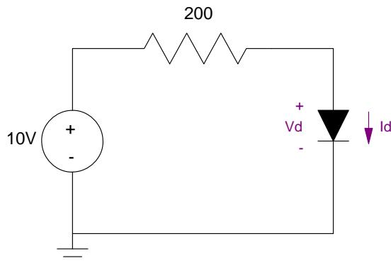
1) Determine the voltage and current through the diode for the following circuit assuming
