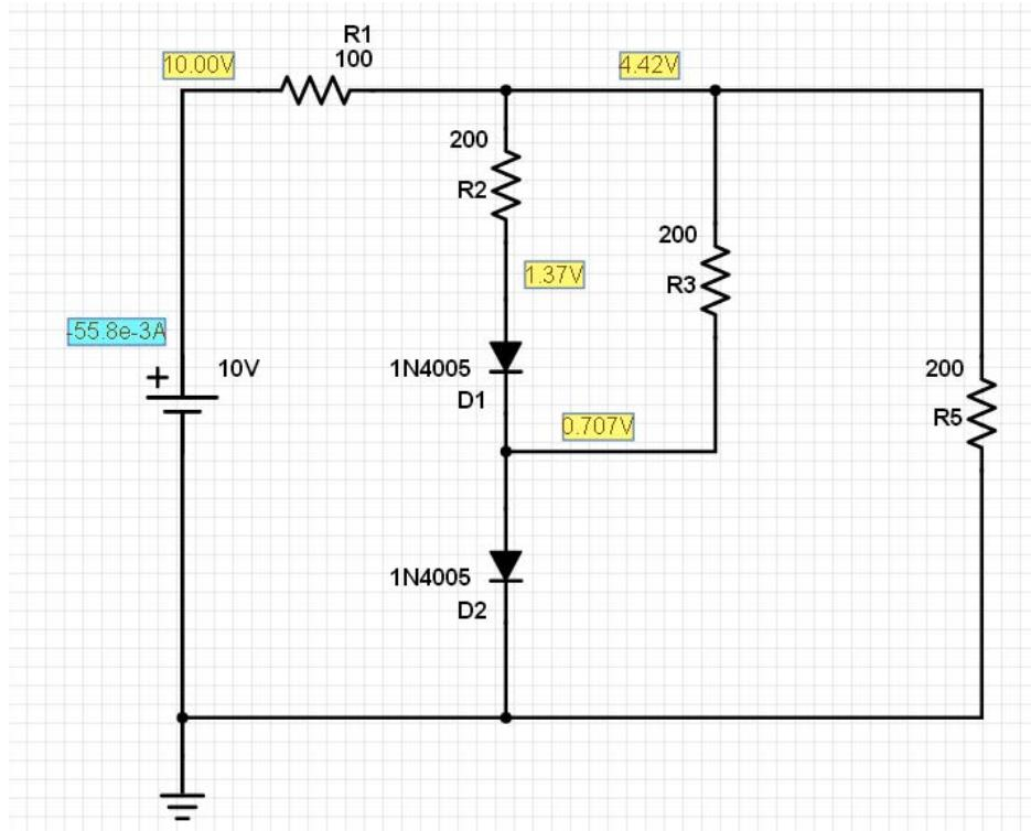
6) In lab, build this circuit using silicon diodes. Measure the voltages and compute the currents
