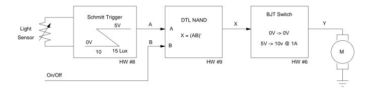
• A, B, X are a 0V / 5V signal capable of driving 1mA
