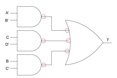
2) Determine a circuit using NOR gates (circle the zeros) for implementing y(t). There are several solutions:
