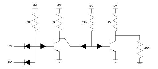
8) Determine the voltages for the following DTL AND gate
