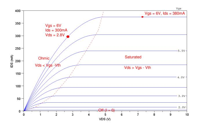
2b) Determine the transconductange gain, kn ( $V_{th} = 1.0V$ ) Pick a point in the Ohmic region
