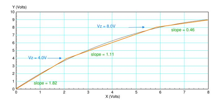
Op-Amp: To get an intial gain of 1.81, add an op-amp with a gain of 1.81
