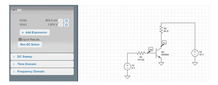
The gain of a 3904 transisor is only 200. This results in the transistor being in the active mode (Vce > 0.2V). If you use two transistors as a Darlington pair, the gain becomes 2002
