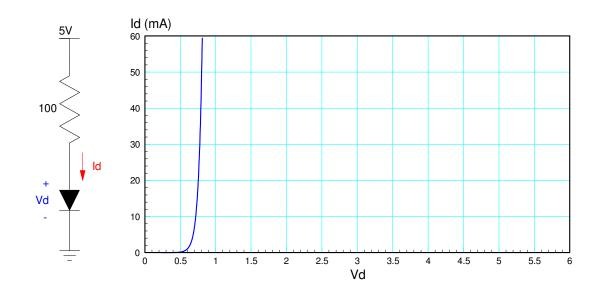
2) Assume ideal silicon diodes (Vf = 0.7V). Determine the voltages and currents
