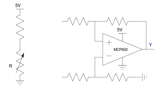
6) Schmitt Trigger: Analysis. Determine the voltages and resistance where the following Schmitt trigger turns on and off. Assume Rx is 1000 + 10\*(Birth Month) + (Birth Day). May 14th gives Rx = 1514 Ohms.
