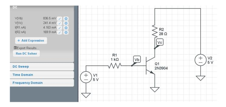
Transistor is On: (Vin = 5V, Vce = 0.241V, Ic = 169.6mA)
