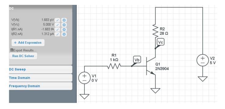
Transistor is Off: Vin = 0V, Vce = 5V, Ic = 0mA (1.31pA)
