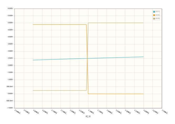
The output switches at 3300 Ohms
