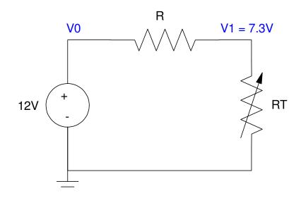
$$V_1 = 7.3V = \left(\frac{R_T}{R_T + 1714}\right) 12V$$
