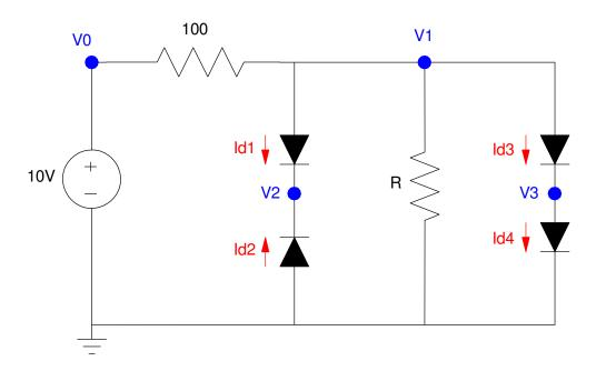
$$I_{d1} = 10^{-11} \cdot \left( \exp\left(\frac{V_1 - V_2}{0.038}\right) - 1 \right)$$
