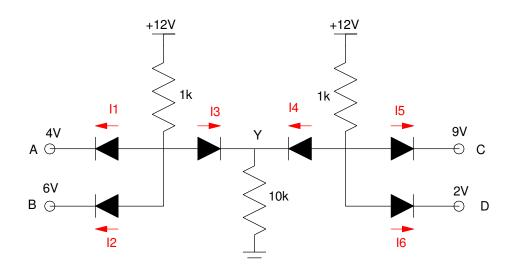
3) Determine the voltages and currents for the following max/min circuit. What function does this circuit implement? Y = f(A, B, C, D)
