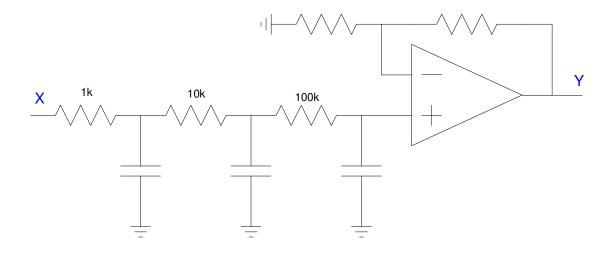
2) Find R and C so that the following filter has the transfer function
