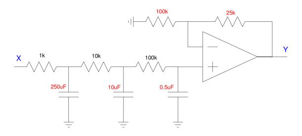
2) Find R and C so that the following filter has the transfer function
