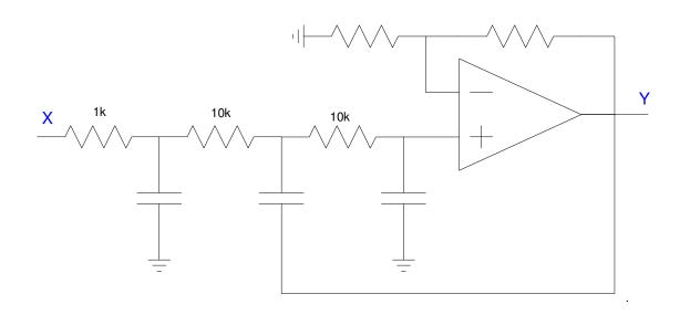
1) Find R and C so that the following filer has the transfer function
