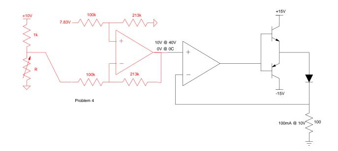
( the PNP transistor in the push-pull amplifier can be deleted - current (and voltage) never goes negative )
