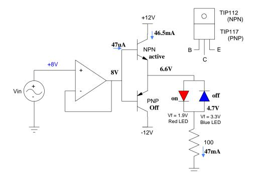
7) Determine the node voltages for the following circuit when the input is -8VDC. Assume a TIP112 and TIP117 transistors.
