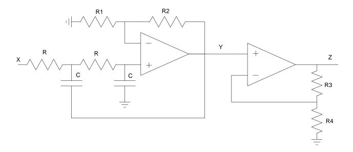
$$Y = \left(\frac{k\left(\frac{1}{RC}\right)^2}{s^2 + \left(\frac{3-k}{RC}\right)s + \left(\frac{1}{RC}\right)^2}\right)X$$
